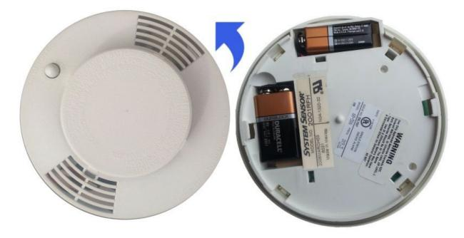
Once you've replaced the batteries, the error on your panel should clear within one hour.
