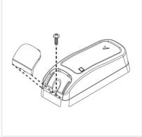
3. Remove and replace the 3-volt lithium CR123A battery.
