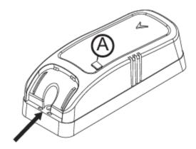
2. Remove the screw and separate the cover from the base
