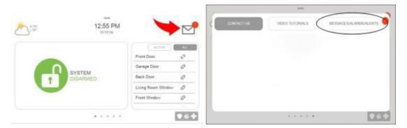
2. Press each alarm to select, or press Acknowledge All, to select all. Press Ok to delete. Then swipe left or right to exit.
